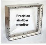
Integrating thin-film resistor sensing and patented air-sampling technology, the Precision Air Flow Monitoring Station features an "air foil" and multiple precision-formed air passages integrated into a stainlesssteel assembly. Built to order, the structure's engineered hole pattern can maintain its measuring accuracy even with 50% hole blockage. Fits into existing ductwork - no duct removal required. NIK PRECISION.
